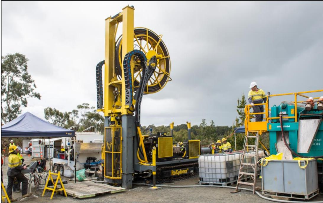
View videos of the the RoXplorer® coiled tubing drilling system
