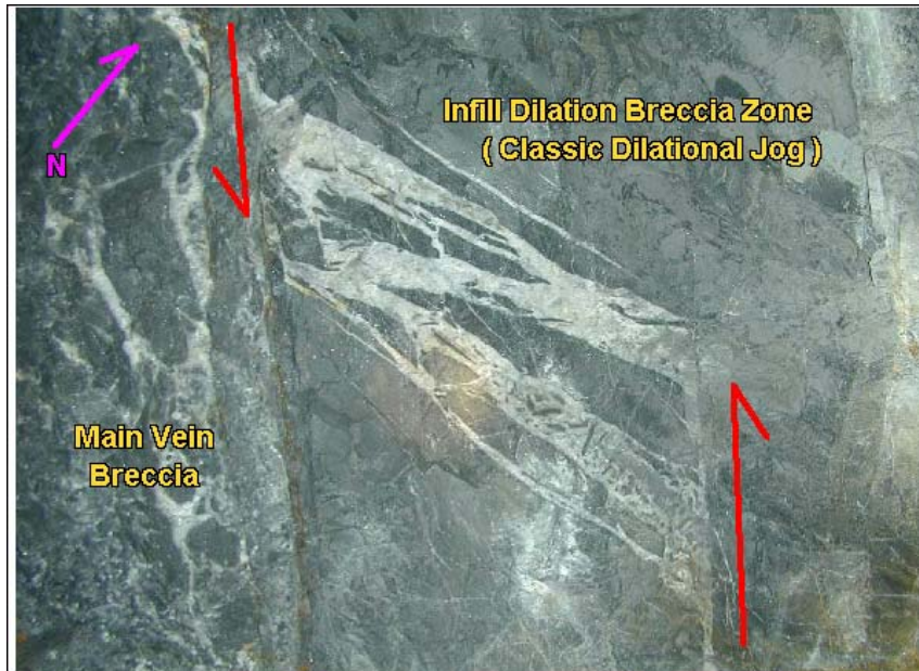
Figure 2: Mineralised structure hosted in dilatational jog, with quartz-stibnite-gold vein infill and adjacent vein breccia zone. Width of image is approximately 1 m.
