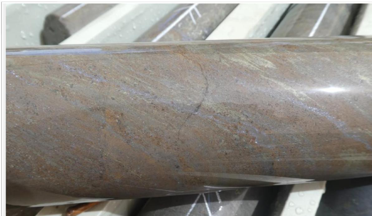
Figure 4: Laminated massive sphalerite, galena, pyrite, hole WTRCDD 192, 358m
