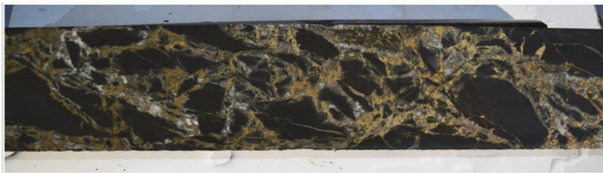
Figure 6: Brecciated silica altered shales with void fill chalcopyrite/pyrrhotite/silica, hole MBDD002, 421.5m.
