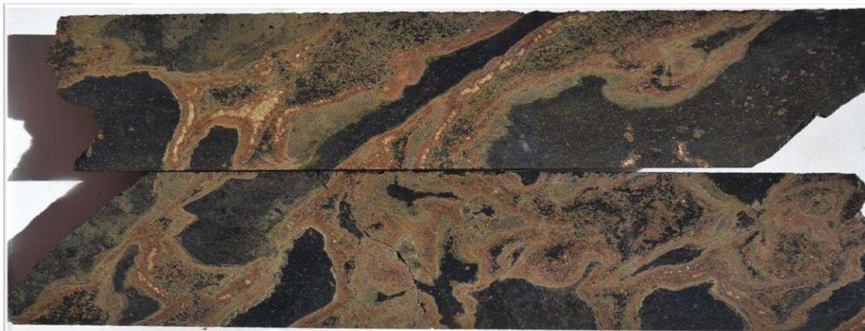
Figure 3: Sphalerite/pyrite stringer veining, hole WTRCDD105, 265-266m
