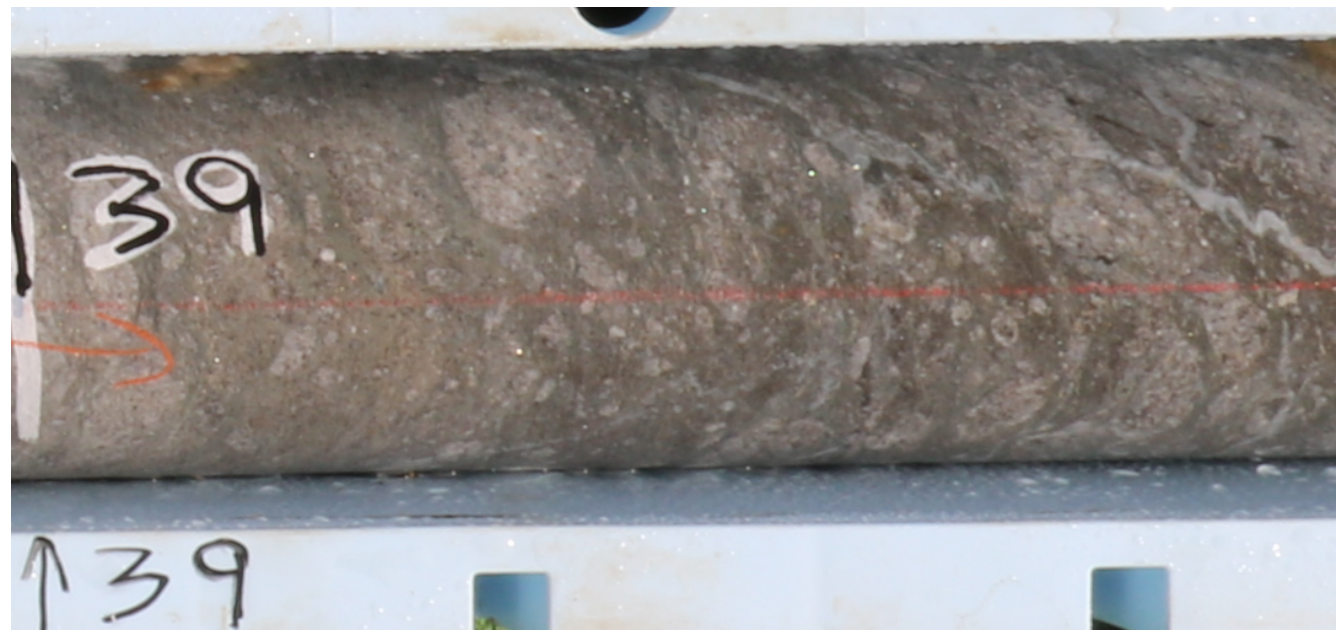
AKDD182 – HQ3 from 35.5m to 35.8m – Volcanic Breccia – angular, ragged, monomict, glassy, rhyolite juvenile clasts hosted in a crystal-rich, quartz-dominated, volcanoclastic sandstone matrix
