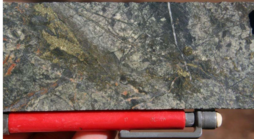
Early chlorite-magnetite alteration cut by later sulphides of a C vein style – DDH 74 248m.
