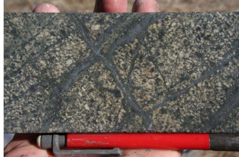
Stockwork B veins in intrusion F DDH 107 214m
