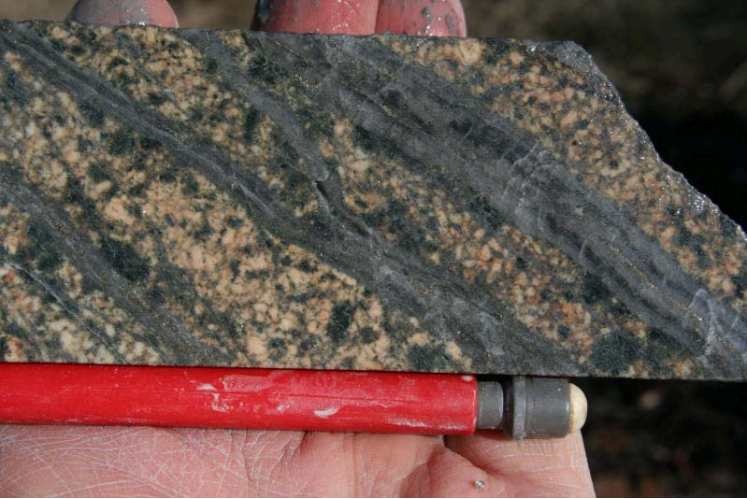
Sheeted laminated quartz-magnetite-sulphide (M style) veins within intrusion F - DDH107, 257 m.
