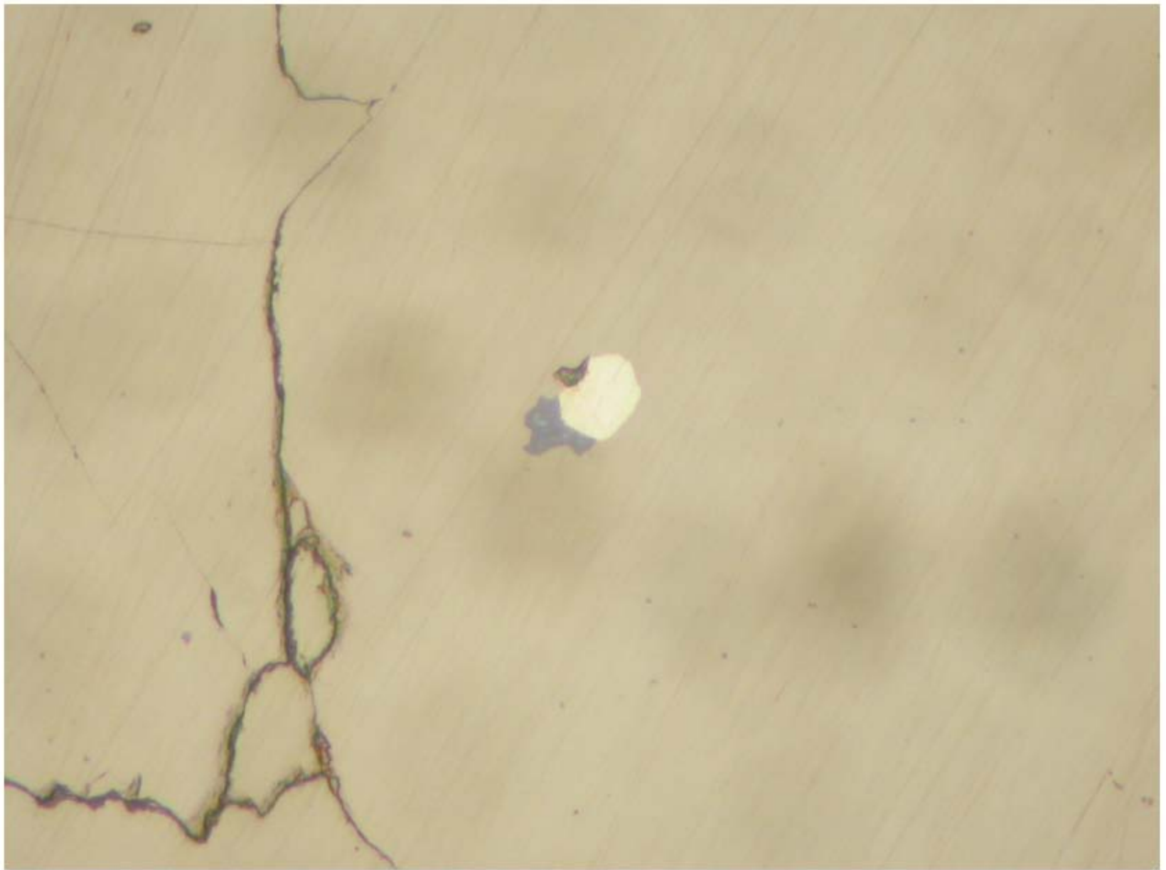
Fig. 42: Portion of coarse chalcopyrite mass with a small composite inclusion of gold (pale yellow) and sphalerite (mid-grey). Gold grain is about 10 microns across. Plane polarised reflected light, field of view ~0.2 mm across.
