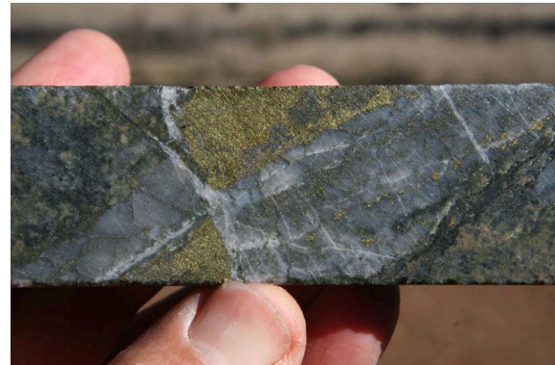
C vein style sulphides overprinting laminated quartz vein - DDH 64 139m
