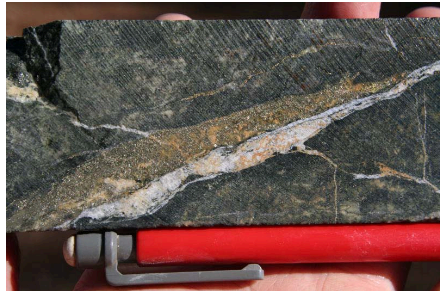
Pyrite-rich D vein with later carbonate - DDH 74 245m
