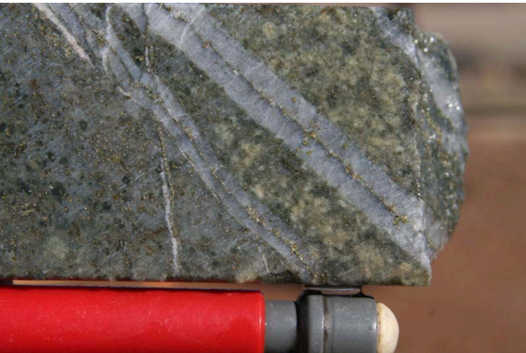
Sheeted B veins in sericite altered intrusion F. Note the central terminations with sulphide fill - DDH 64, 132m.
