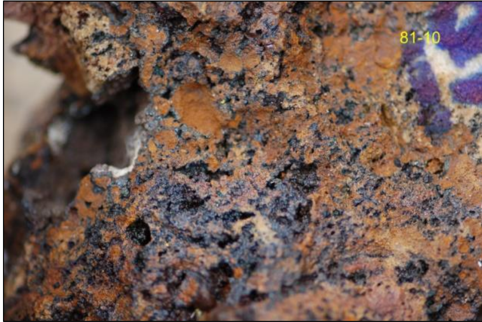
Figure 4. La Sorpresa, vuggy silica and Fe oxide: sample 81-10 reported at 8.6 ppm Au, 1790 ppm As (see Appendix 1)
