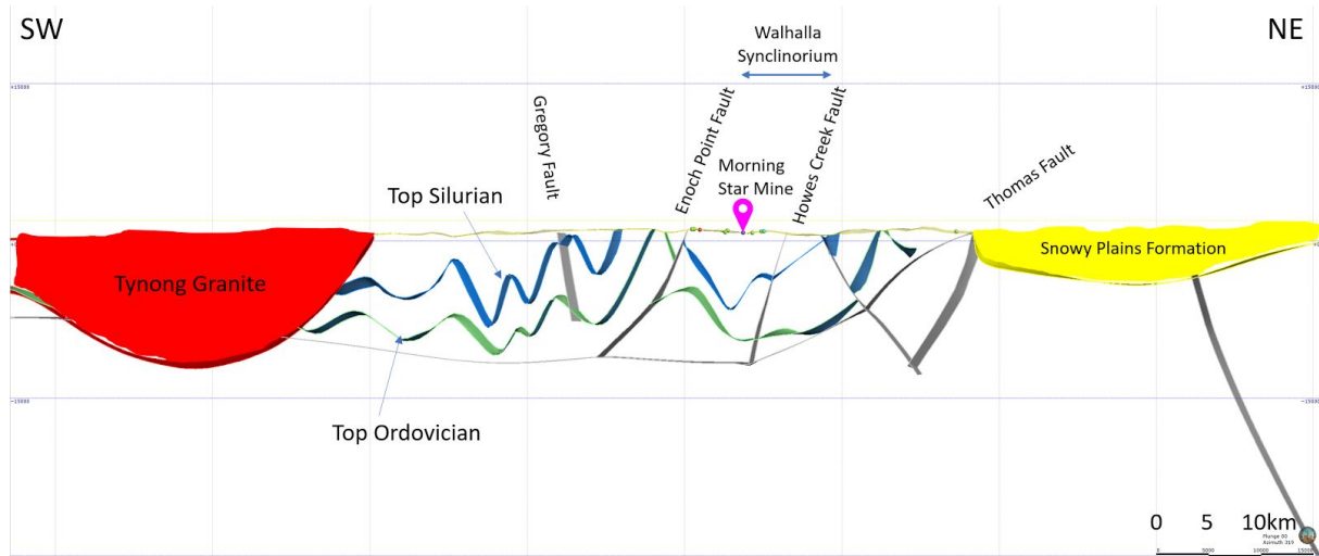
Fig. 2. Cross section extracted from the Melbourne Zone 1:250,000 3D model of McLean et al (2010), showing the position of the Morning Star mine on the southwest-dipping limb of the Walhalla Synclinorium
