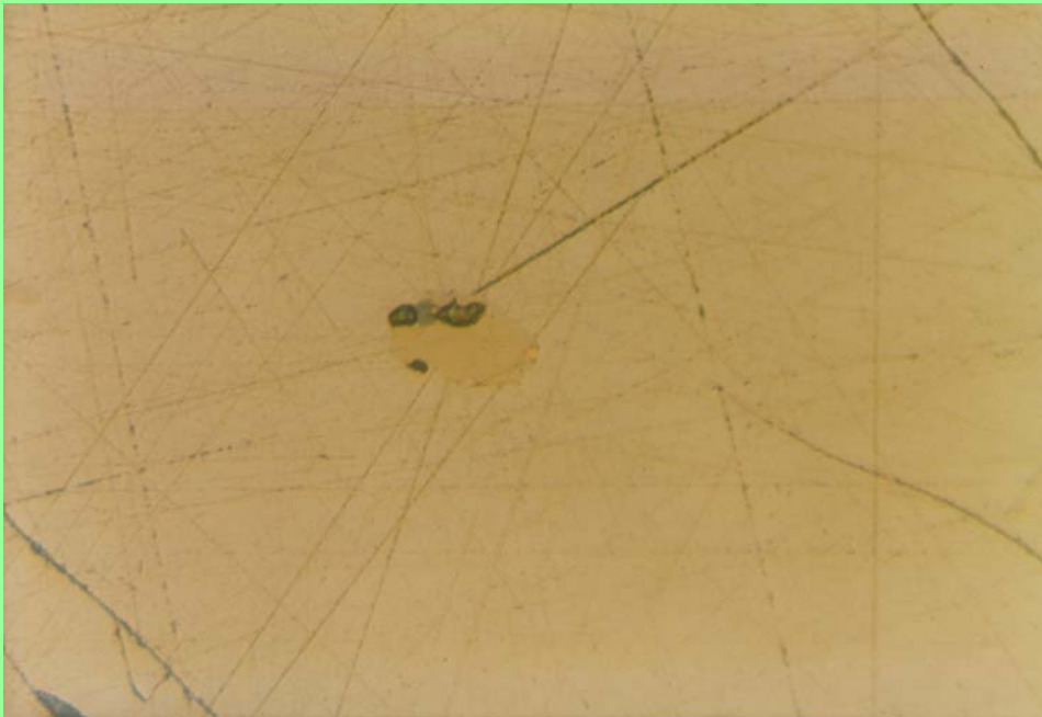
A rounded chalcopyrite inclusion with a small gold grain in pyrite WD15 236.5m WOV 0.27mm
