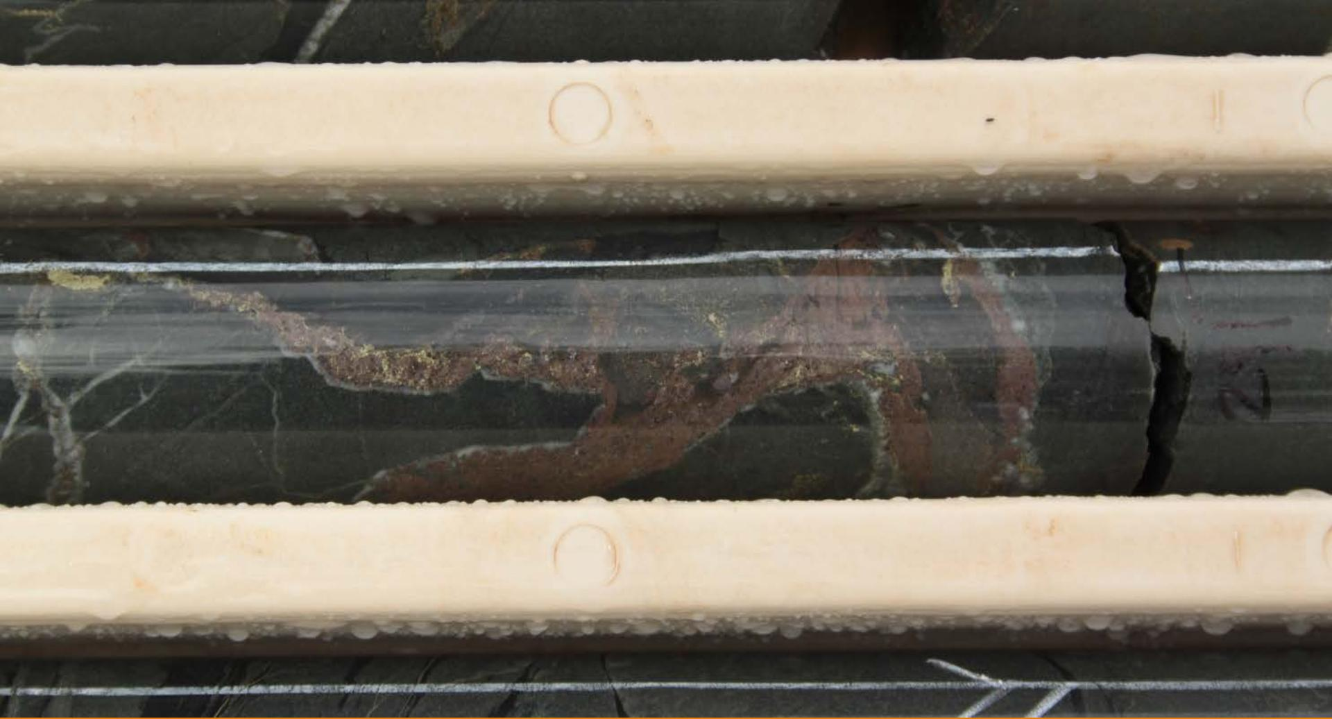
Stringer sphalerite/pyrite/galena veining in upper Shume Formation. Hole 4MRCDD010: ~291m
