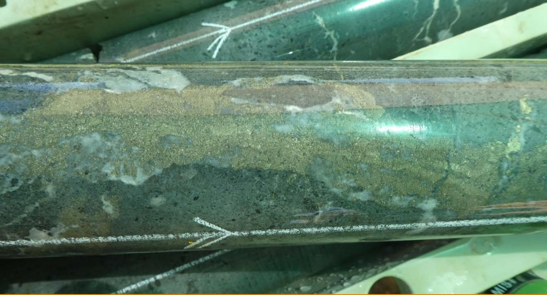
Stringer chalcopyrite/pyrite/silica veining, lower Vivigani Formation, hole WTRCDD188: 442m.
