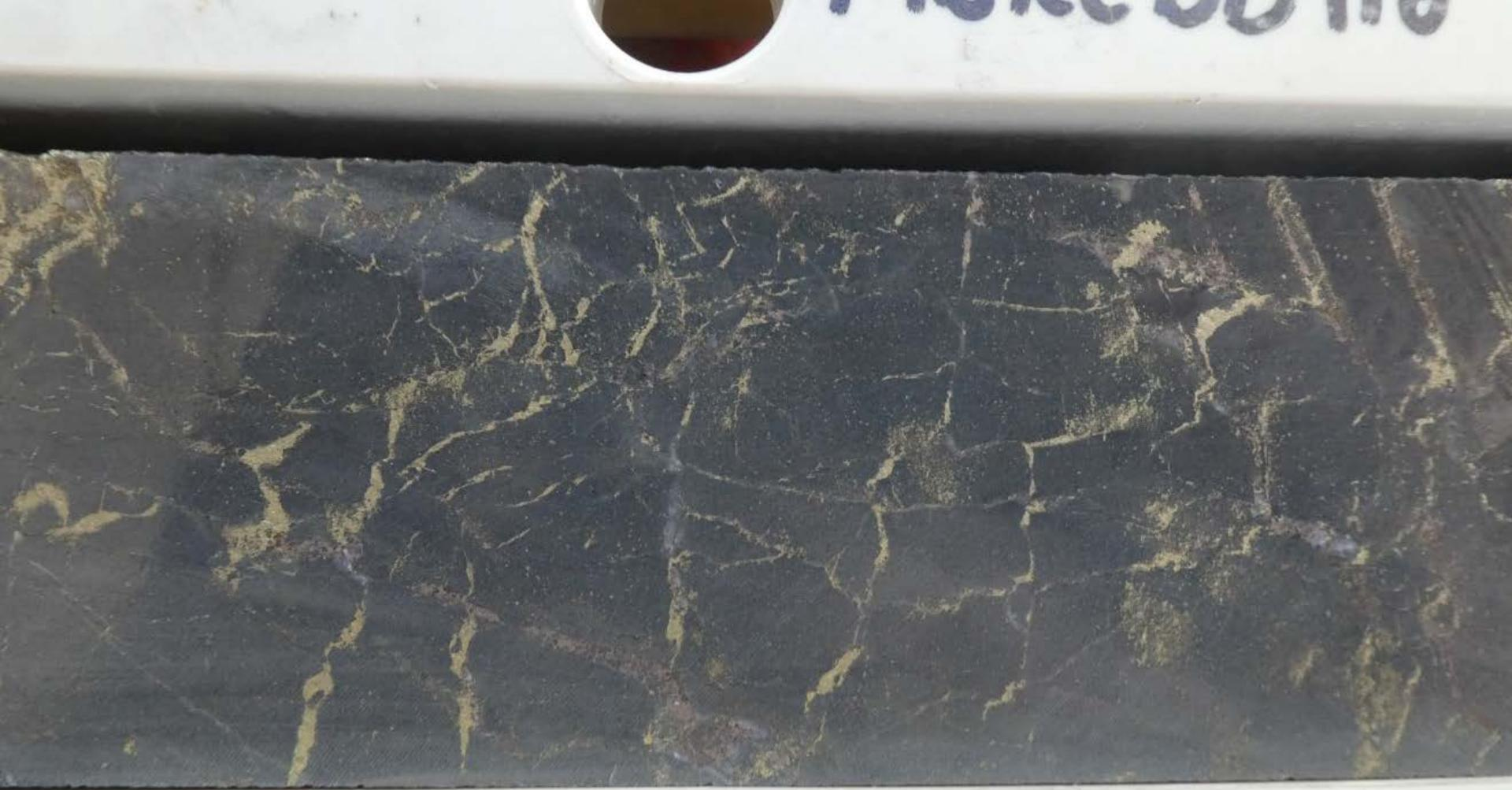
Crackle brecciated silica altered Shume Formation shales,
