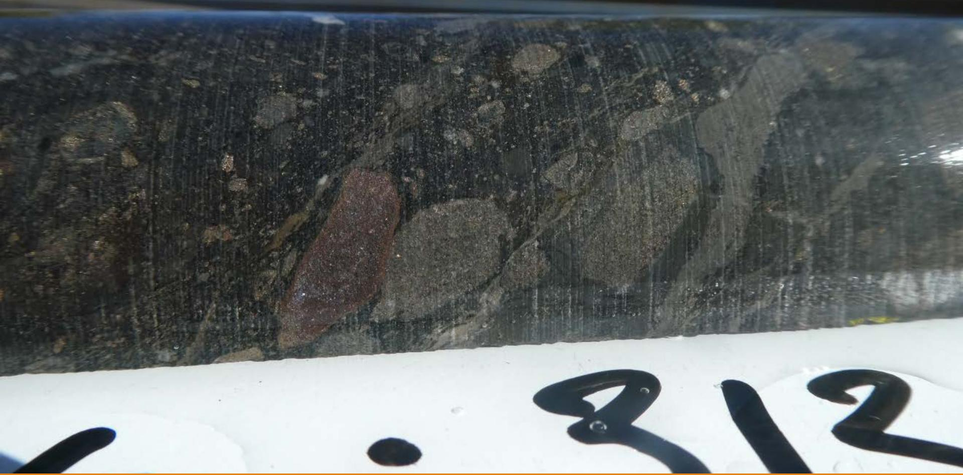
Rafted Zn/Pb sulphide clast in volcaniclastic breccia, MBDD024:
