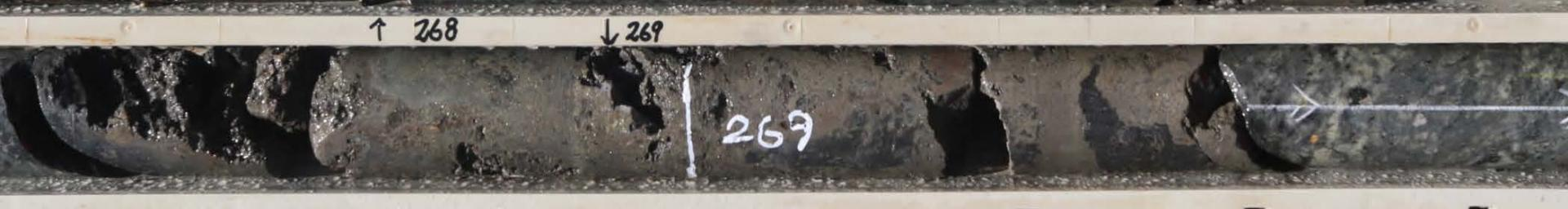
Sphalerite/pyrite stringer veining
