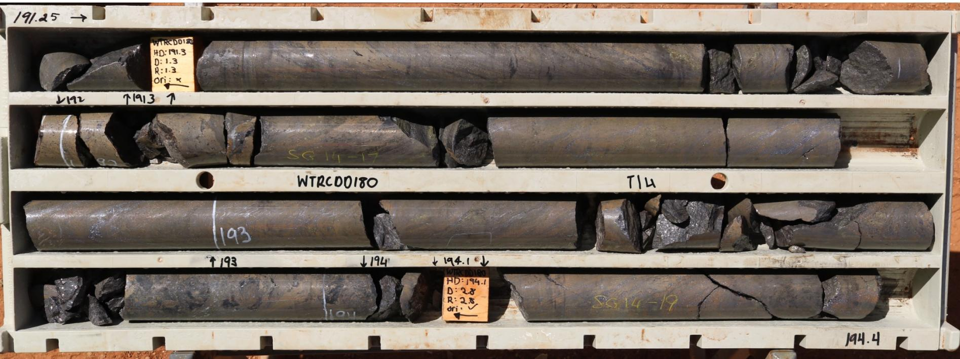
Very high grade laminated and brecciated massive sphalerite/galena/pyrite, basal Wagga Tank Formation
