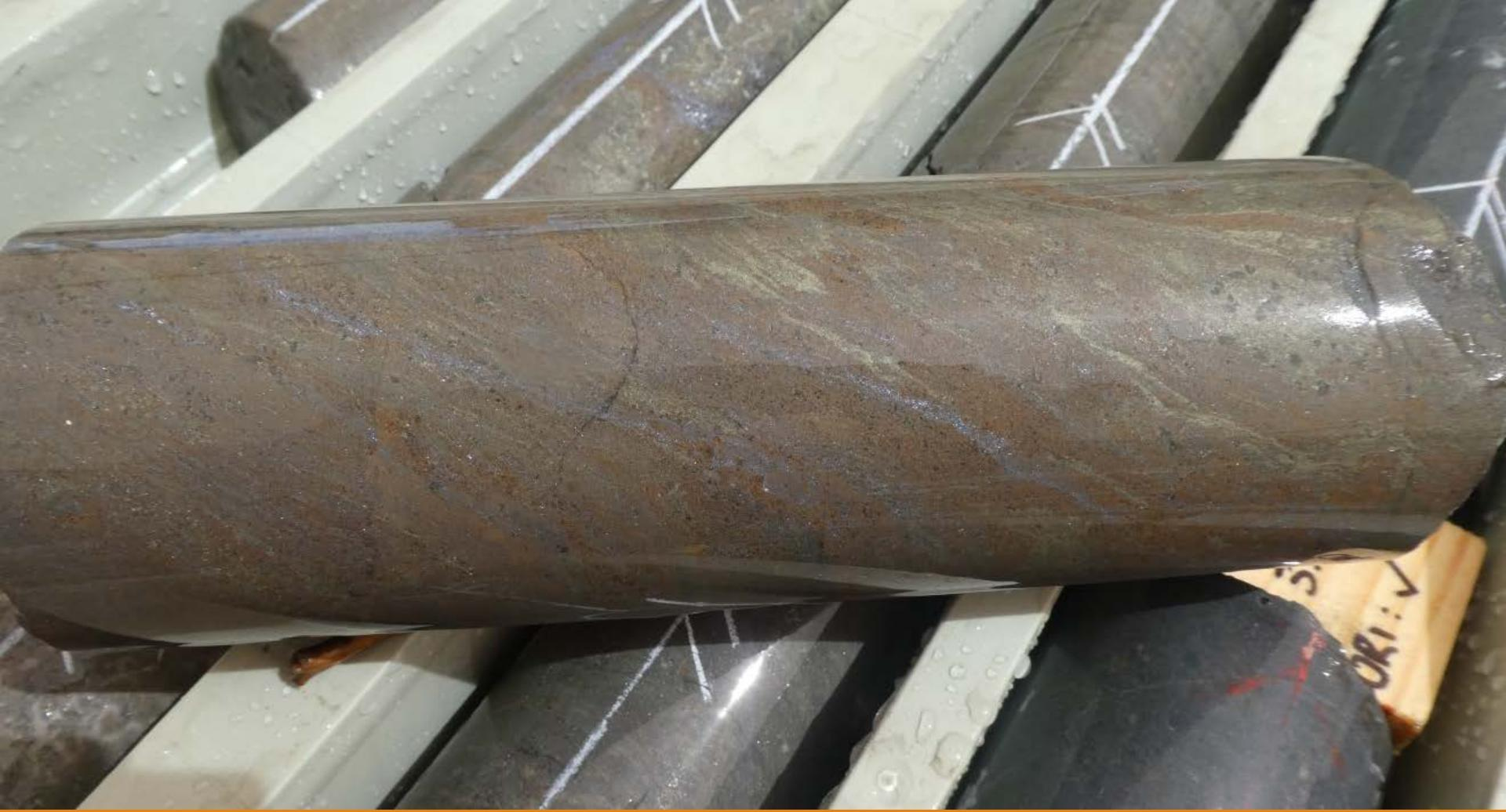
Laminated sphalerite/galena/pyrite, Vivigani/Wagga Tank contact, hole WTRCDD192:~358m
