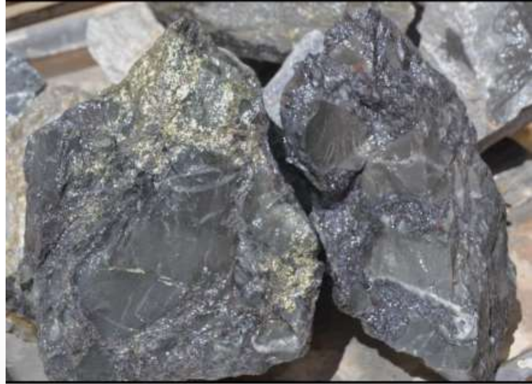
Samples of strong zinc-lead and copper sulphide mineralisation from the first cross cut into the Hera ore body
