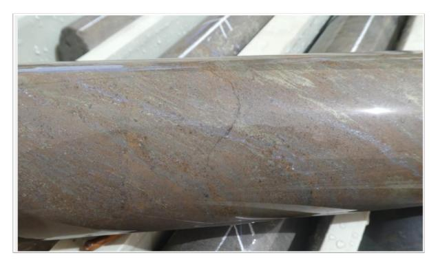
Figure 4: Laminated massive sphalerite, galena, pyrite, hole WTRCDD 192, 358m
