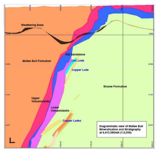
Figure 5: Mallee Bull diagrammatic cross section 6413380N
