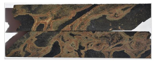
Figure 3: Sphalerite/pyrite stringer veining, hole WTRCDD105, 265-266m
