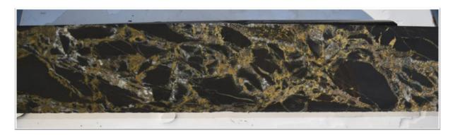
Figure 6: Brecciated silica altered shales with void fill chalcopyrite/pyrrhotite/silica, hole MBDD002, 421.5m.
