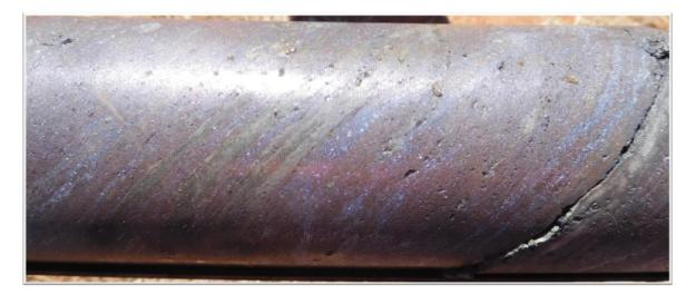
Figure 7: Laminated massive sphalerite, galena, pyrite, hole MBDD028, 85m.
