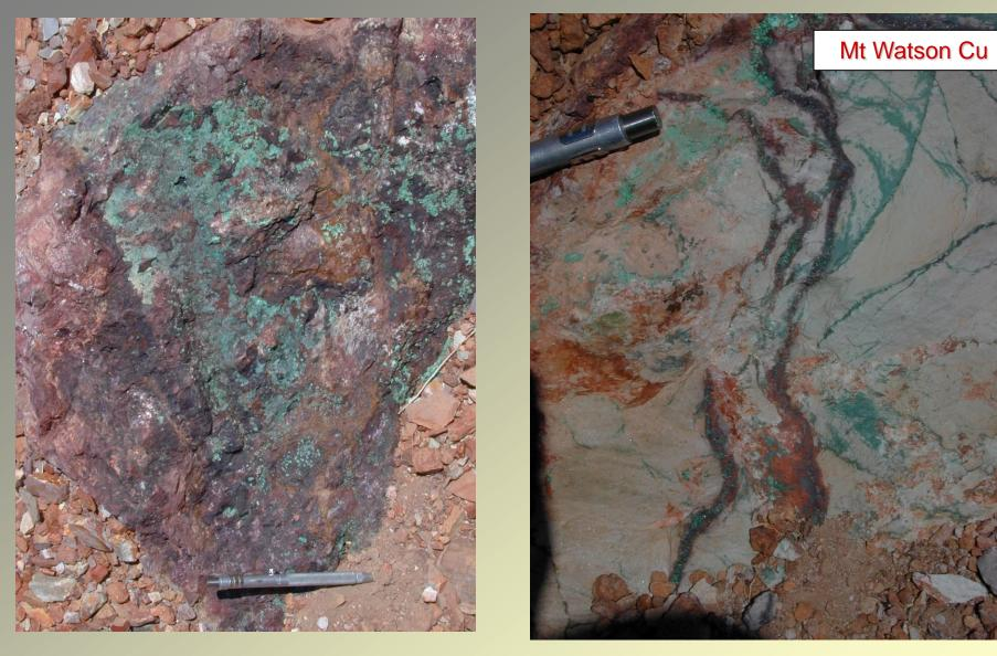
Typical oxidised vein mineralisation trucked 25km to SXEW plant at the old Mt Cuthbert operation
