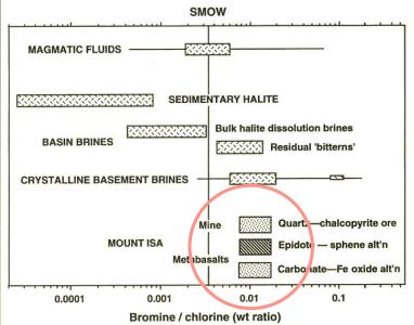
FIG. 9. Neutron activation analyses of Br/Cl in inclusion-bearing quartz samples, in comparison with Br/Cl ranges of some modern fluids (summary from Heinrich et al., 1993).
