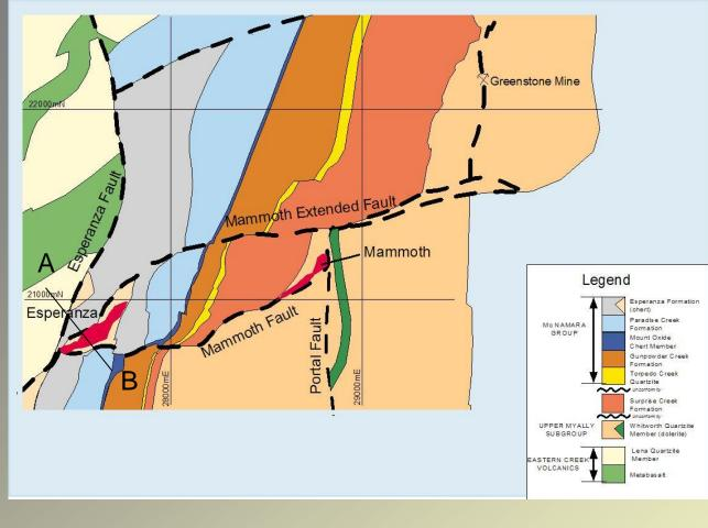
Esperanza was difficult to drill because of the massive chert cap to the main orezone; Sillitoe considered it to be an epithermal deposit; chert could also be due to leaching of carbonates and collapse in weathering domain.
