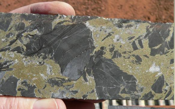
Brecciated grey ?carbonaceous siltstone with py-cpy sulphide breccia
