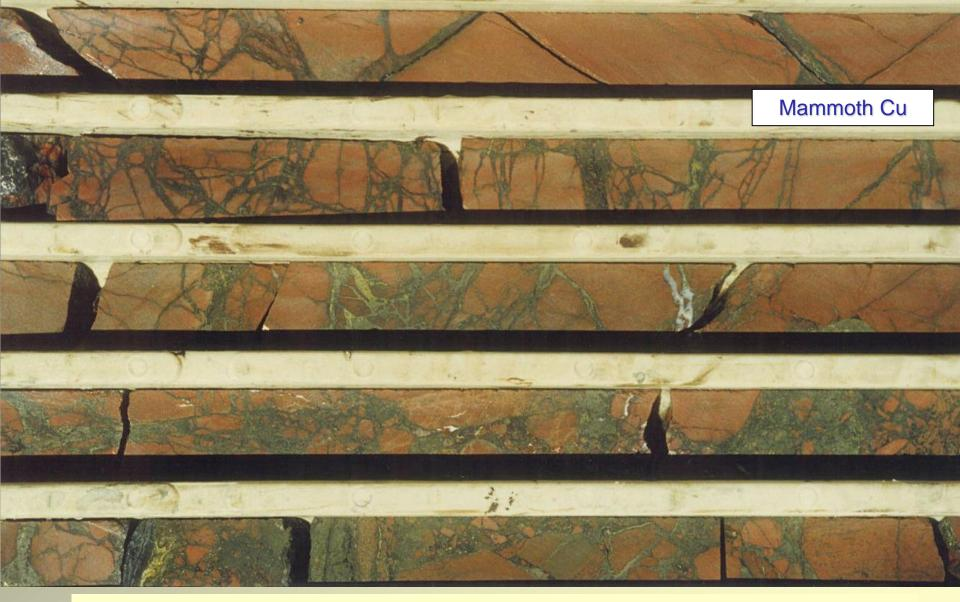
Mammoth D3 Cu – progressive hydrothermal fracturing in brittle massive pink feldspathic quartzite of Myally Sugroup; density of fracturing ranges from clast supported (top) to matrix-supported (base); sulphides mainly py, minor cpy and chalcocite.
