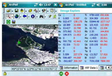
Streaming XRF Meta-Data into ArcPAD Mobile GIS
