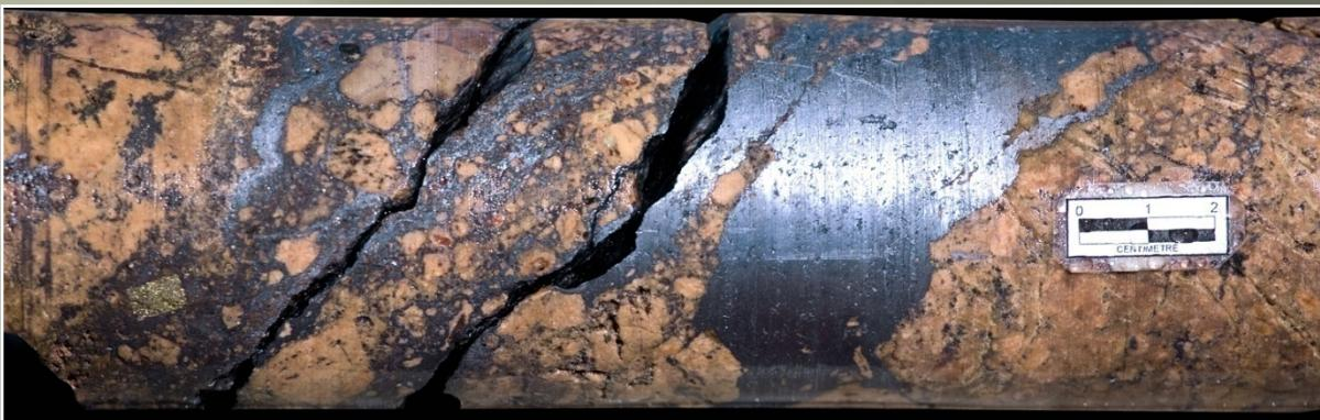
MDQ0147 - Breccia, sheared sediment with Molybdenite in filling fractures.
