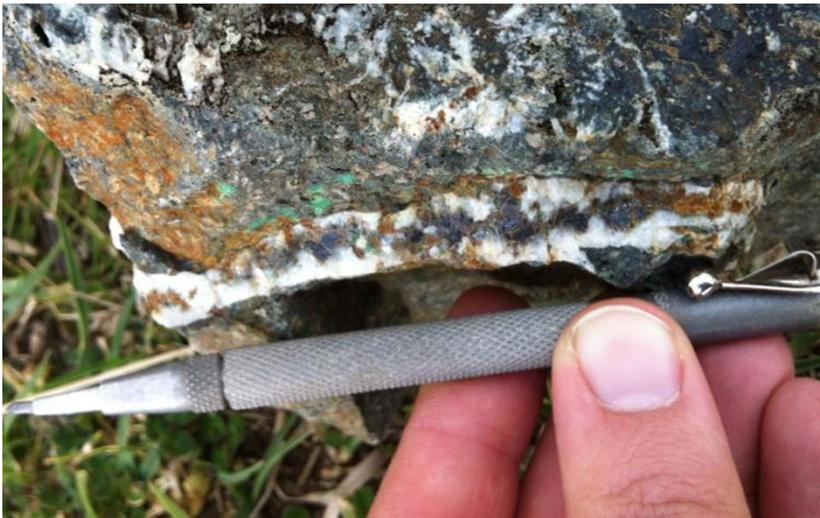
Quartz-carbonate veining with malachite and bornite at Fitzroy mine
