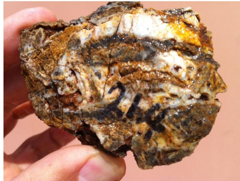
*Right: Epithermal style quartz vein (D vein?); and top right: Fe/Mn fracture fill*
