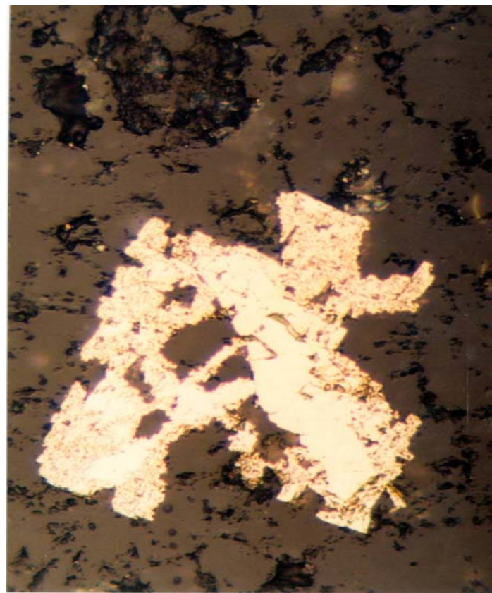
Coarse grained pyrite in silicified sediment with pitted, etched and partially dissolved rims, that are overgrown by very fine grained poorly crystalline arsenean pyrite. Field of view 0.3 mm
