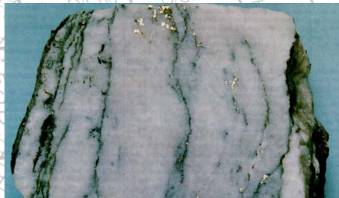
Ribbon quartz vein and gold – Blackwater mine
