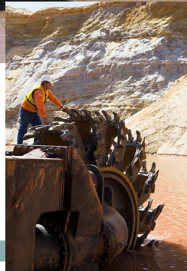
Spud dredge with cutter raised 2009
