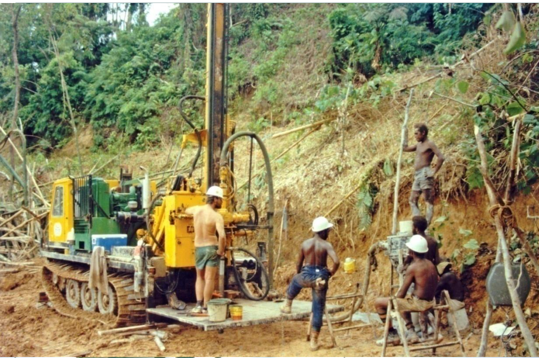
Track mounted reverse circulation air core drill, c1987
