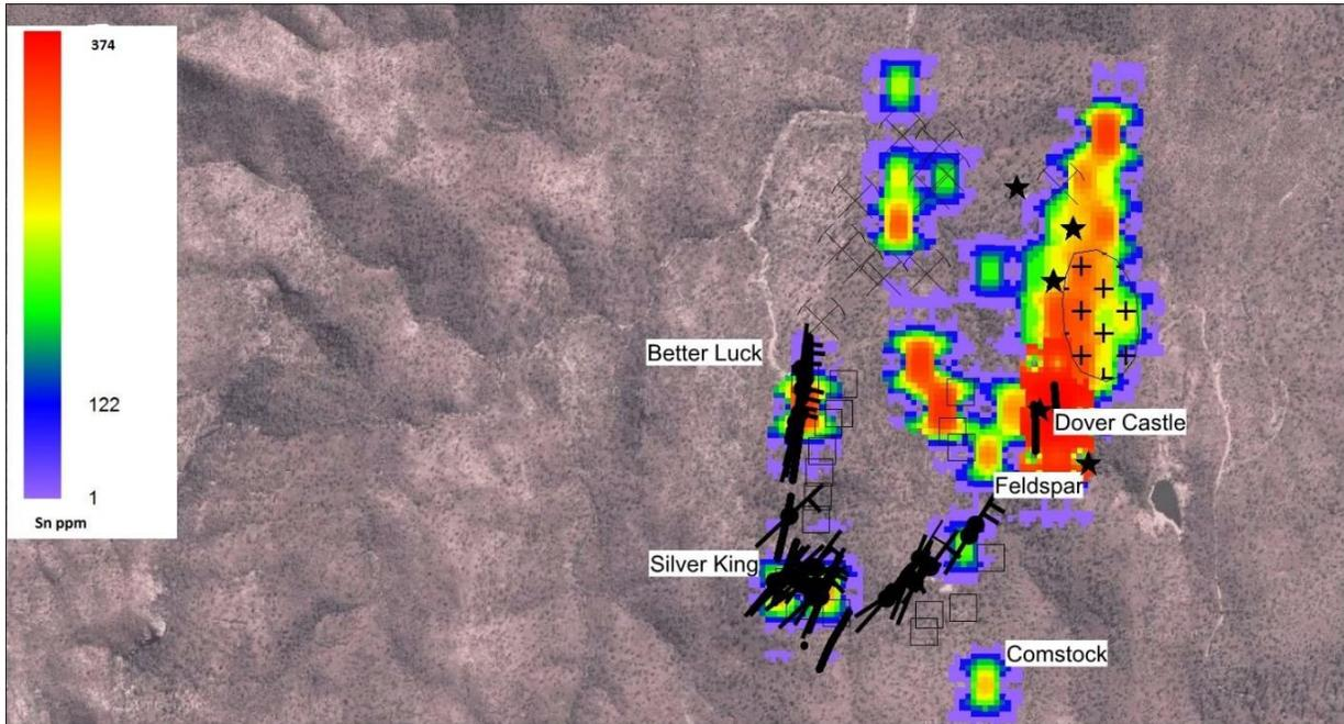
Figure 13. Gridded Sn in soils on a satellite image overlain by Dover Castle Metals RC drill holes (squares), Houston Oil and Minerals drill holes (black stars), interpreted vein orientations (black lines), historically worked pits (black crosses) and Dover Castle porphyry outcrop (cross hatch) (Menzies 2014c).
