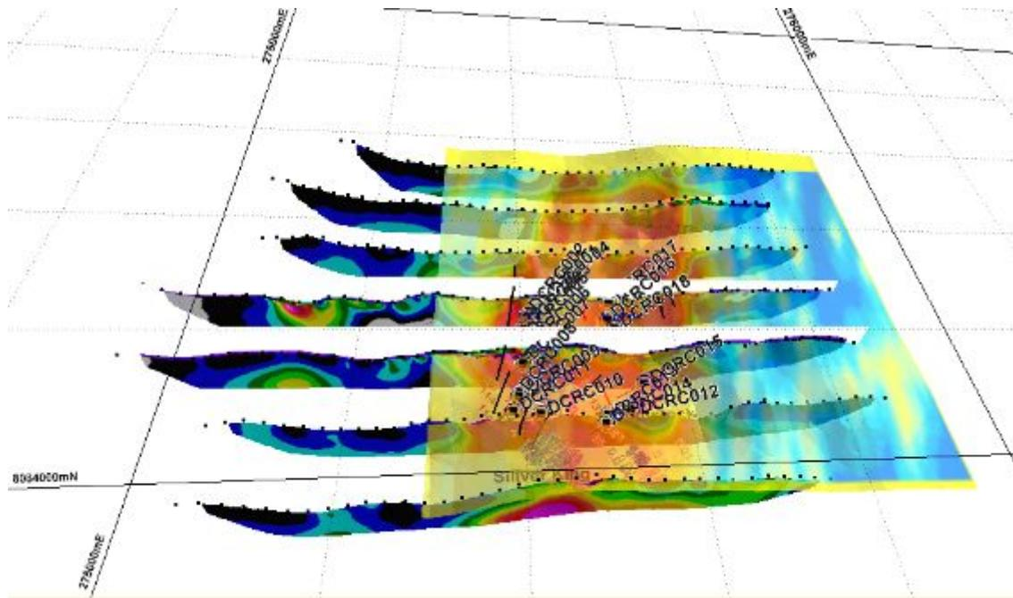
Figure 15. Gridded Pb in soil overlain on chargeability pseudo sections with orange > 329 ppm Pb (Menzies 2014c).
