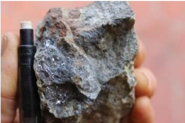
Plate E. Massive galena and red-brown sphalerite which reported 0.12 g/t Au, 423 g/t Ag, 1.4 % As, 0.3 % Cu, 3130 ppm In, 14.4 % Pb, 16.9 % Zn Comstock prospect.
