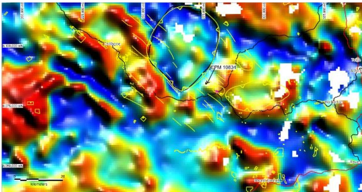
Figure 4. First vertical derivative bouguer gravity data (Geoscience Australia) overlain by aeromagnetic interpretation (yellow lines) showing the location of EPM10834 (Menzies, 2014b)
