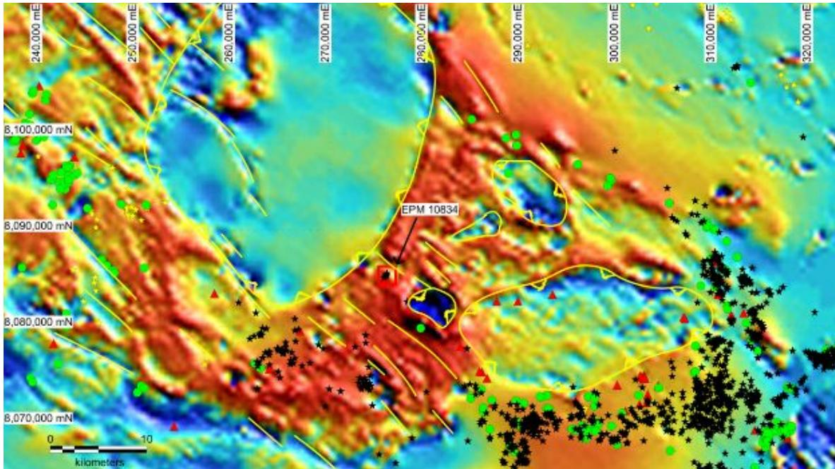
Figure 3. Total magnetic intensity aeromagnetic data (Geoscience Australia) showing a prominent low to the NW, E and NE of EPM 10834 (Dover Castle), NW trending faults (yellow lines) and mineral occurrences (yellow stars = Au, red triangles = Ag, green circles = Cu, and black stars = Sn) (Menzies, 2014b)
