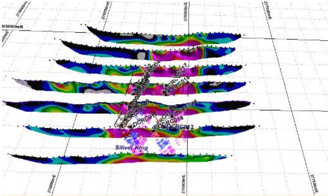
Figure 8. 3D model of induced polarisation chargeability pseudo sections (purple is >12.09 mV/V) and previous Dover Castle drill holes (Menzies 2014c).
