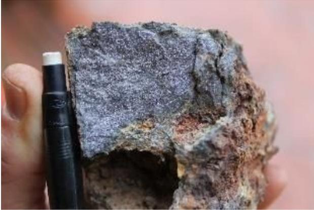
Plate A. Massive galena-quartz ± carbonate which reported 5030 g/t Ag, 783 ppm As, 604 ppm Cu, 147.5 ppm In, 58.5 % Pb, 1.0% Zn from Better Luck prospect.
