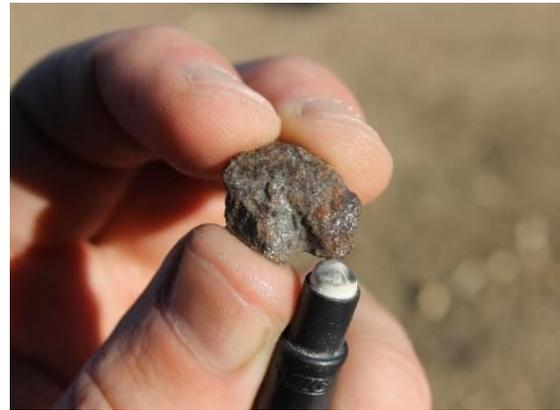
Plate D. Galena, dark brown sphalerite and pyrite mineralisation which reported 1m at 163 g/t Ag, 30.2 ppm In, 3.6 % Pb, 1.8 % Zn from 89-90m in DCRC001 drilled into Better Luck prospect.
