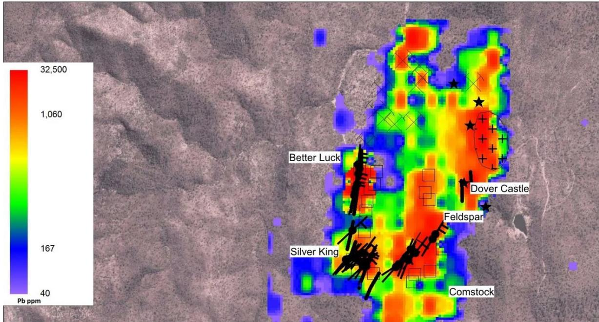
Figure 11. Gridded Pb ppm in soils on a satellite image overlain by Dover Castle Metals RC drill holes (squares), Houston Oil and Minerals drill holes (black stars), interpreted vein orientations (black lines), historically worked pits (black crosses) and Dover Castle porphyry outcrop (cross hatch) (Menzies, 2014c).
