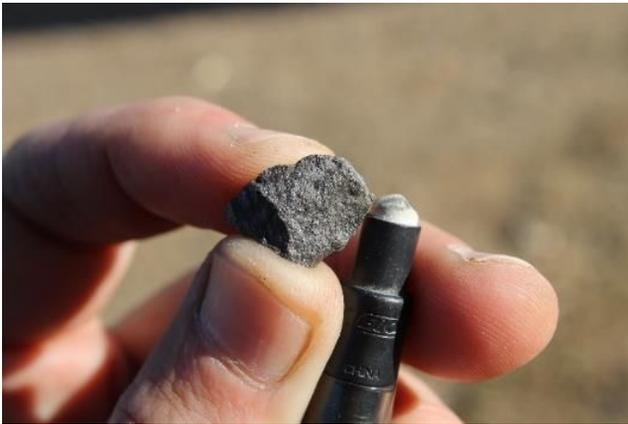
Plate C. Massive fine-grained galena-sphalerite-pyrite, which reported 1m at 797 g/t Ag, 154 ppm In, 15.25 % Pb and 8.2 % Zn from 87-88m in DCRC001, drilled into Better Luck prospect.
