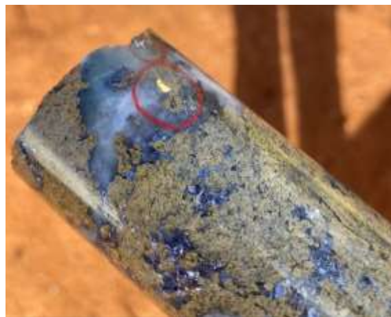
Federation drill core with very coarse-grained gold to 4mm (circled) associated with massive low-iron sphalerite (light brown), galena (metallic grey) and quartz (white) from FDD085. This sample is a part of a one metre interval grading 59.5% Pb+Zn and 137g/t Au.
