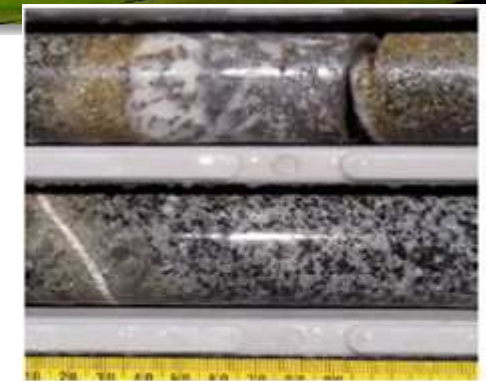
SGRDD033: closest to the potential causative blind pluton; encountered a wide mineralised zone in altered granodiorite over 27.35m downhole (from 11.75 - 39.1m) comprising narrow sulphide bearing alteration veins with anomalous gold, the highest grade vein 19.2 g/t Au over 0.16m (top core row).
