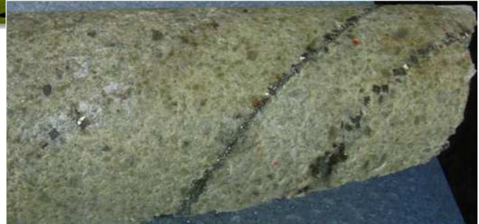
Martins Shaft: SGRDD003, sheeted sulphide veins (3mm wide, euhedral pyrite and arsenopyrite) in phyllic altered felsic dyke
