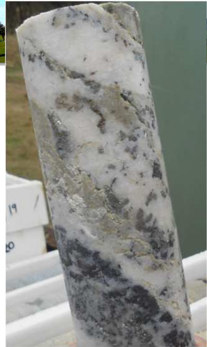
Martins Shaft: SGRDD004, 19.6 g/tg Au, 2.18oz/t Ag, 0.64%/t Sb from 58m (HQ core, diameter 63.5mm). Vein filling composed of abundant carbonate (calcite), plus crudely banded and disseminated medium to coarse grained sulphides, minor, but locally abundant fine-grained sericite and a little quartz.
