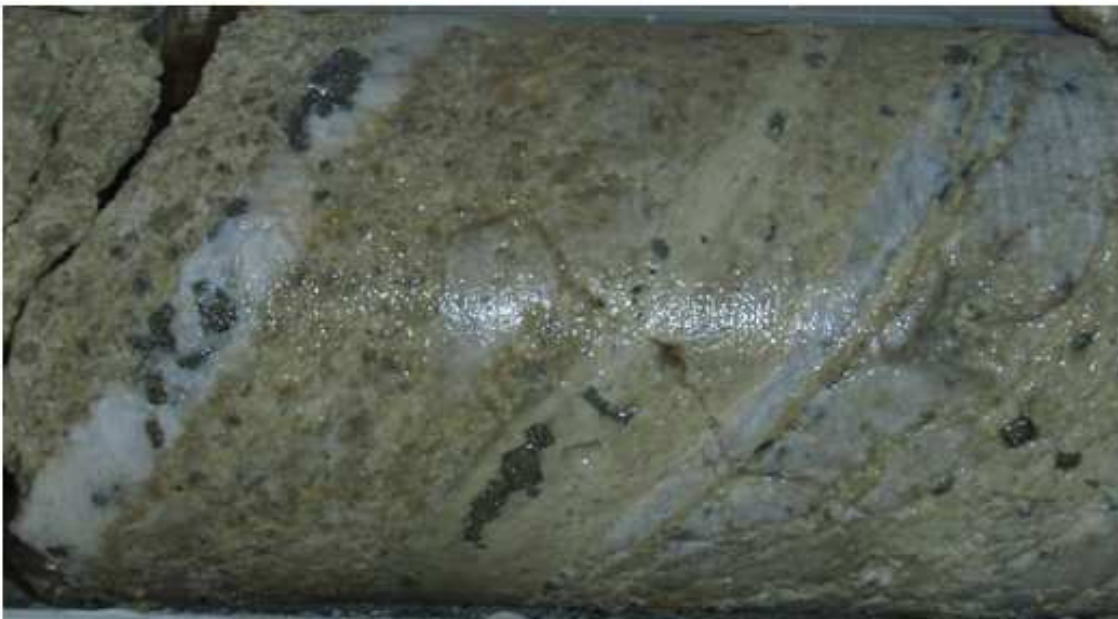
Martins Shaft: SGRDD002, close-spaced sheeted, carbonate-quartz-pyrite-arsenopyrite veins in phyllic altered felsic dyke (around 27m). 27-28m, 10.5 grams/tonne gold, 13.35 grams/tonne silver (HQ core, diameter 63.5mm).
