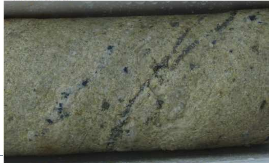
Martins Shaft: SGRDD002, sheeted sulphide (arsenopyrite, pyrite) veins (2-4mm wide) in phyllic altered felsic dyke (around 26m)
