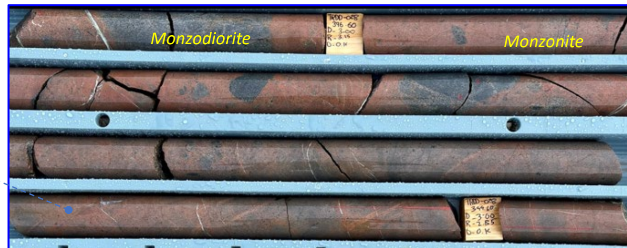
ABOVE: Monzonite (red-orange) with monzodiorite xenoliths (grey): TRDD028 at 395m
