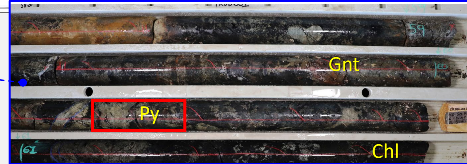
TOP - TRDD001: Garnet (Gnt)-chlorite (Chl) skarn with semi-massive pyrite, disseminations of chalcopryite, chalcocite and native copper within 51m @ 1.17 g/t Au, 0.54%Cu from 39m, including 20.5m @ 1.94 g/t Au, 1.18%Cu from 57.6m.
