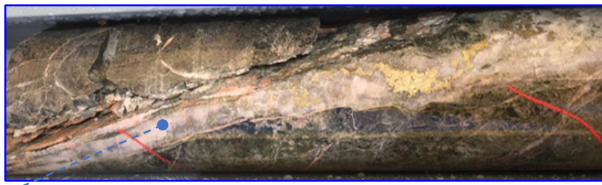
TOP - TRDD029 @ 510m: Carbonate-quartz vein with chalcopyrite, hosted by volcaniclastic rocks, occur above the Upper Skarn
