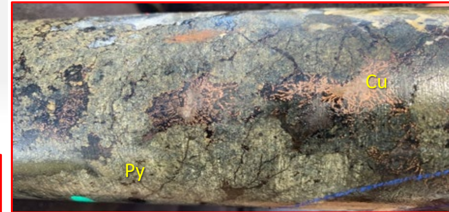
BOTTOM - TRDD001: Semi-massive pyrite (Py), disseminations of chalcopryite and native copper (Cu) in a skarn zone from TRDD001 with 1m @ 4.24 g/t Au and 1.6 %Cu from 60.6m.
