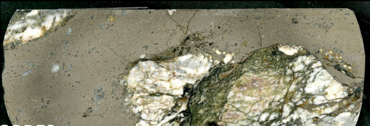
Massive pyrrhotite – cassiterite replacement of dolomite, Renison Bell Sn mine, Tasmania
