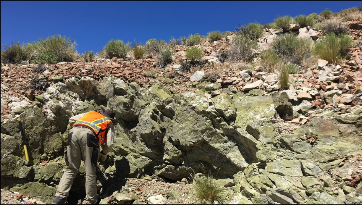
Massive epidote skarn cut by calcite veins with chrysocolla coatings, Yerington, Nevada
