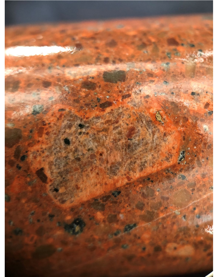
Bornite rimming chalcopyrite within compositionally zoned K-feldspar megacryst in quartz monzonite porphyry – E22 Deposit (Photo: R. Lesh)
