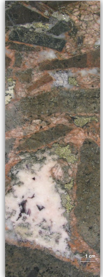
K-feldspar – pyrite – chalcopyrite – calcite – fluorite cemented breccia
