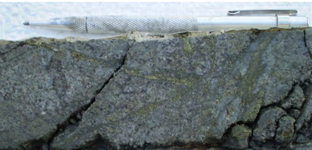
WR321: Diss and veined chalcopyrite, 1m at 0.7g/t Au and 2.1% Cu, 955m
