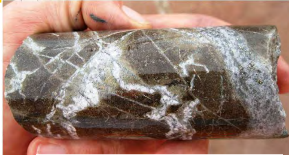
WR321: 762.5m Biotite altered metasediments with quartz-chalcopyrite bearing (~1%) veins
