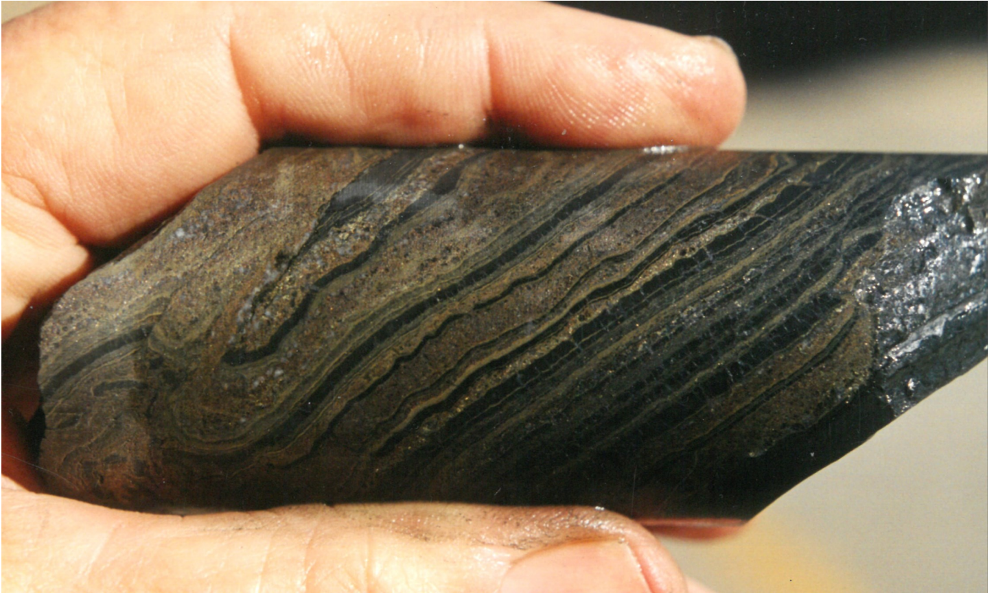
GF2001-9: D orebody, top to left; banded pyritic siltstone with sphalerite bands. Some fold crenulation—Z-type fold with shearing in fold axial zone, with coarser sulphide breccia.
