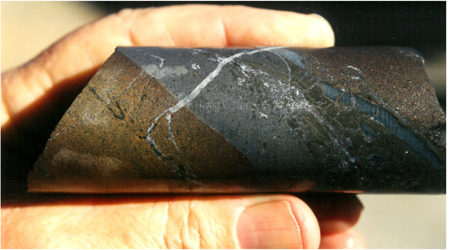
GF2001-5: Massive banded sulphide, E orebody—sphalerite and galena, plus late ?calcite vein; uphole to left. Getting close to D orebody (i.e. towards HW)
