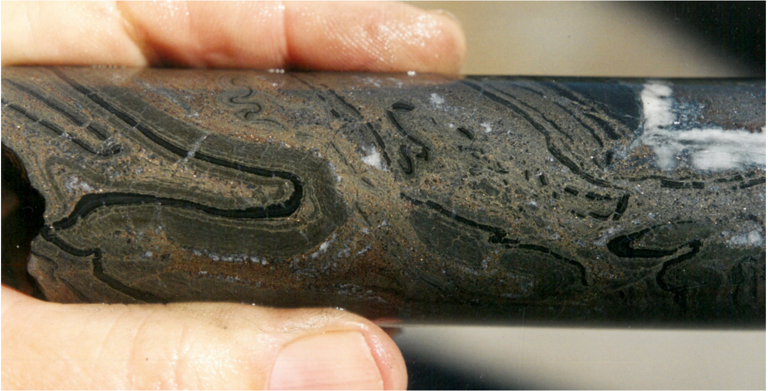
GF2001-1: Part of C orebody—top to left. Folded and brecciated banded pyritic siltstone with red-brown sphalerite. Many mobilised sulphide-shale breccia zones with fold remnants
