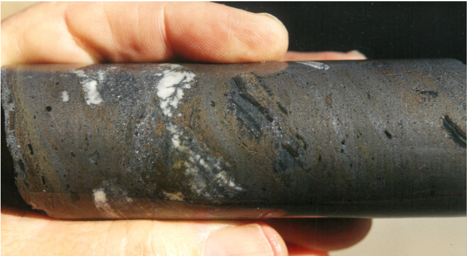
GF2001-8: D orebody, top to left., Massive sulphide breccias, crudely layered—galena and sphalerite, and late ?calcite veining. Breccia contains fragments of bedded siltstone
