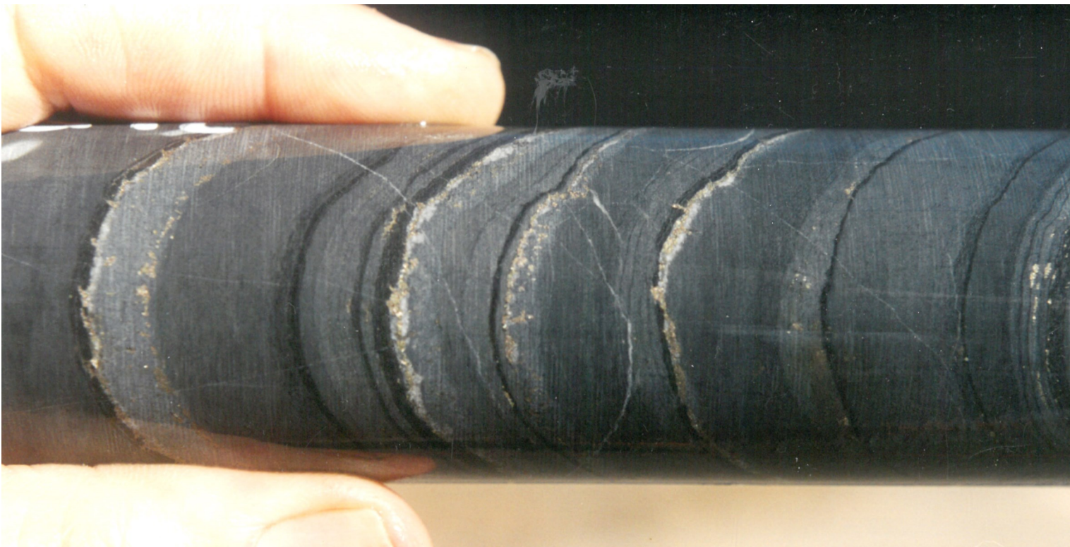
GF2001-6: Near top of E orebody. Rhythmically banded cyclic sedimentation, top to left (towards HW). Cycles are from thicker-bedded basal grey dolomitic siltstone, then lighter pyritic carbonate zone then thin dark shale
