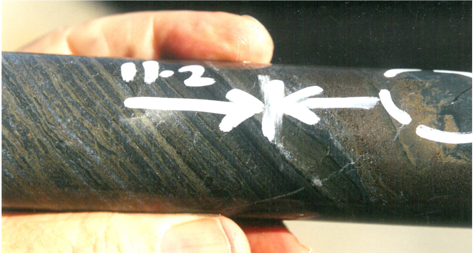
GF2001-4: E orebody— pyritic dolomitic siltstone with sphalerite to right, and possible tuff marker bed ??
