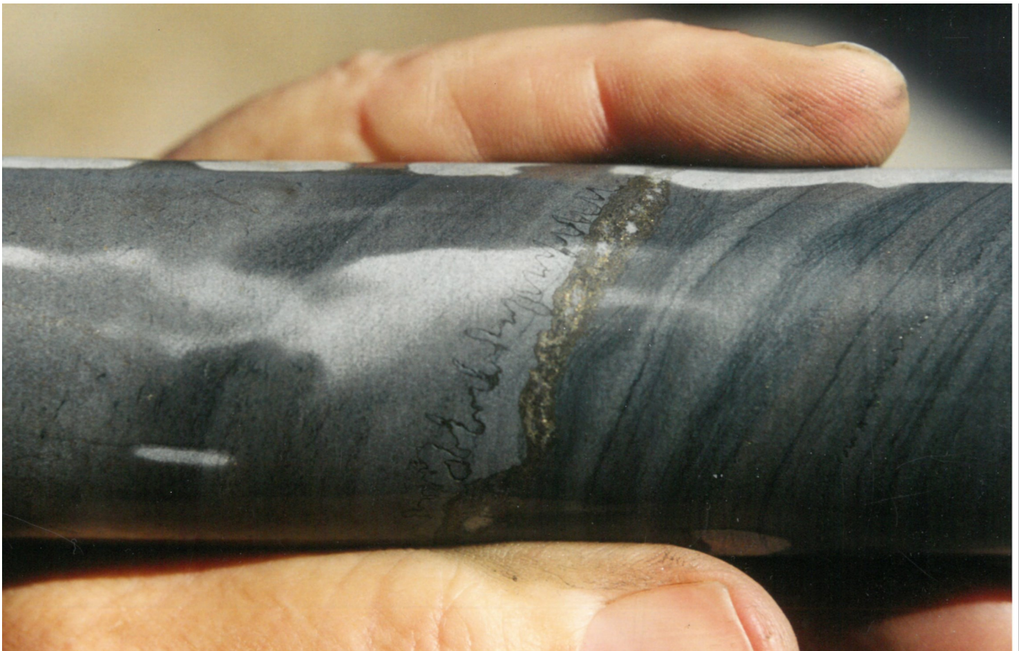
GF2001-12: Top of C orebody, top to left, dip steep to west. Barren dolomitic siltstone with notable stylolites, minor pyrite. Part of the Urquhart shale.
