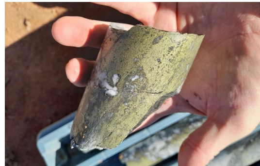
Figure: KSNDH015 - 71.9m: Chalcopyrite vein. Sample interval 71.6m to 72.3m: 5.5% Cu, 0.5g/t Au, 13g/t Ag.
