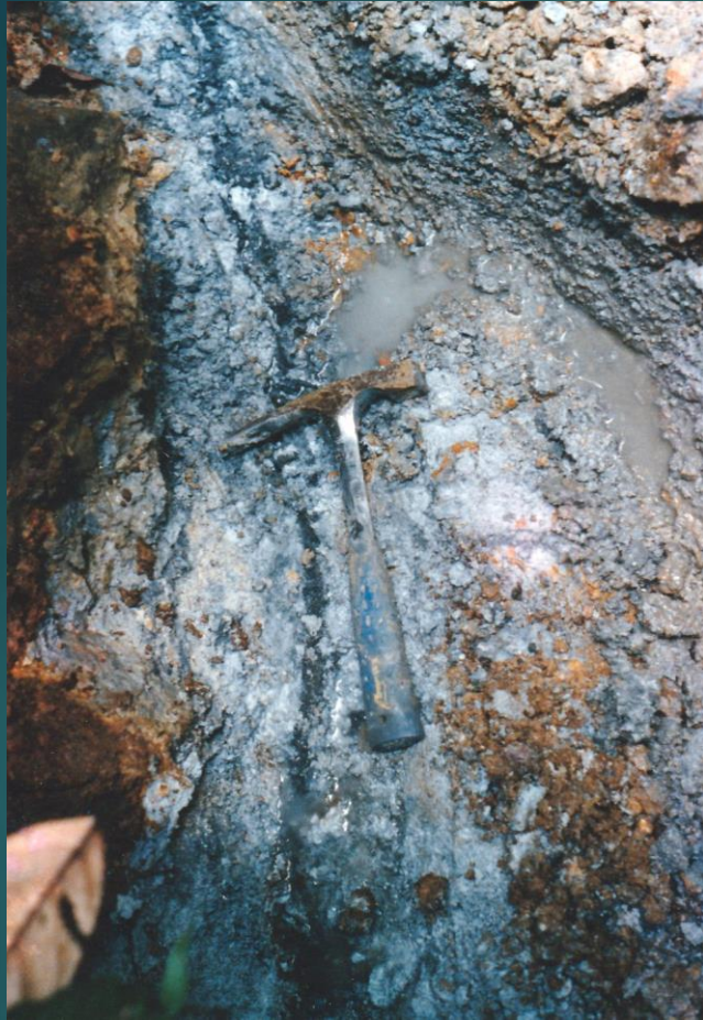
Base-metal vein in soft, argillic-altered diorite
