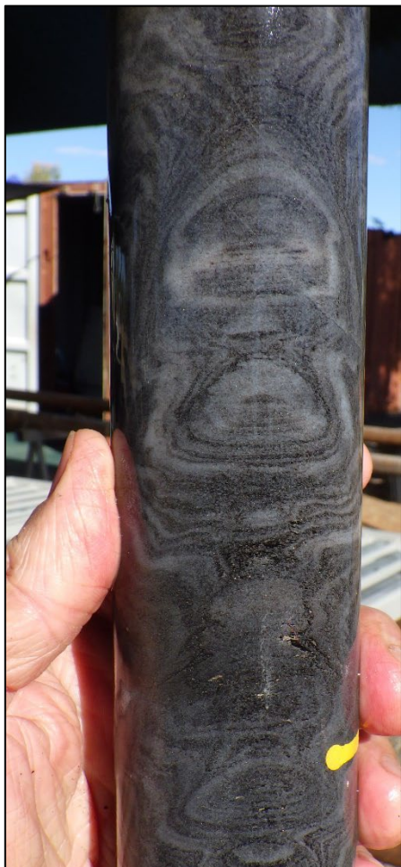
Type 2 Mushroom interference fold patterns. N-S F1 overprinted by F2 E-W shortening
