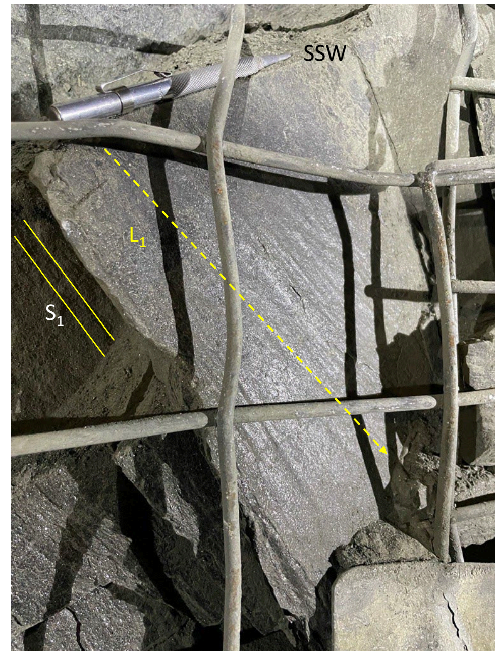
Pervasive foliation with lineation in eastern mineral corridor
