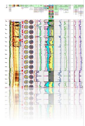
By integrating wireline logging measurements, an accurate determination of rock type can be made. This information can be used to determine stress orientation and magnitude, as well as estimate mechanical rock properties.
