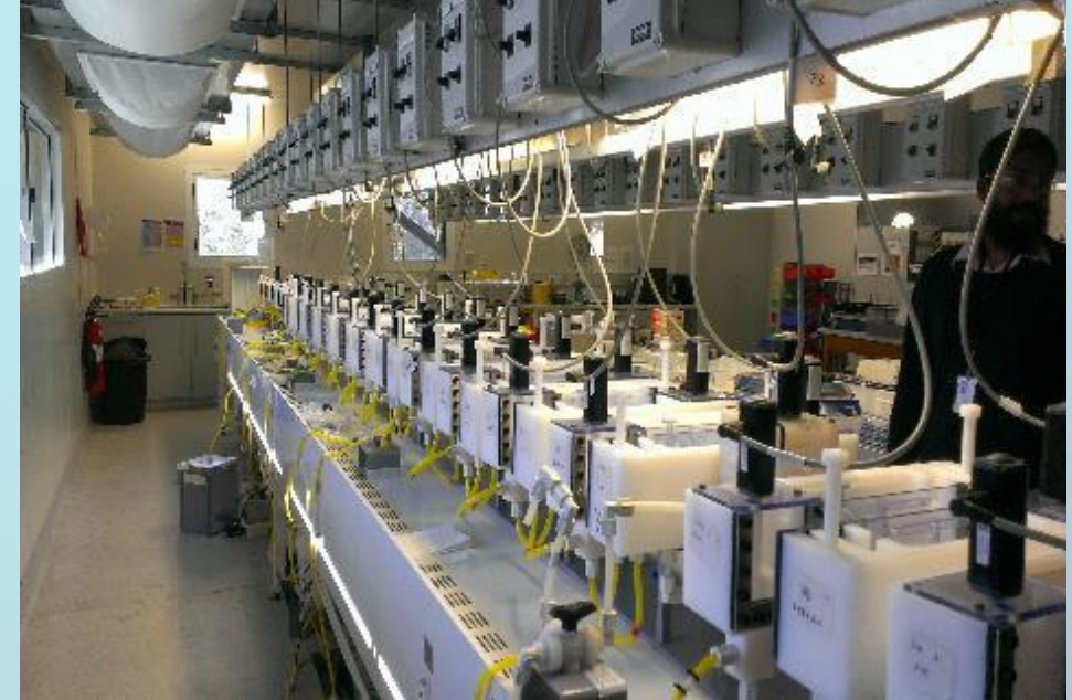
The hafnium zirconium solvent extraction and separation circuit (a world first)
