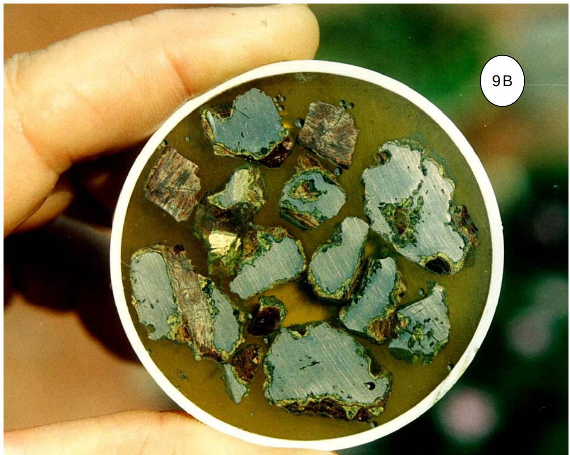
Figure 9A,B: Group of native bismuth nuggets; 9a shows natural state of nuggets recovered by metal detector from eluvium; nuggets show iron-stained exterior; 9b shows nuggets in epoxy mount slabbed for polishing and examination; note metallic nature of bismuth locally with pinkish reflection, and green oxidised rind (bismutite).
