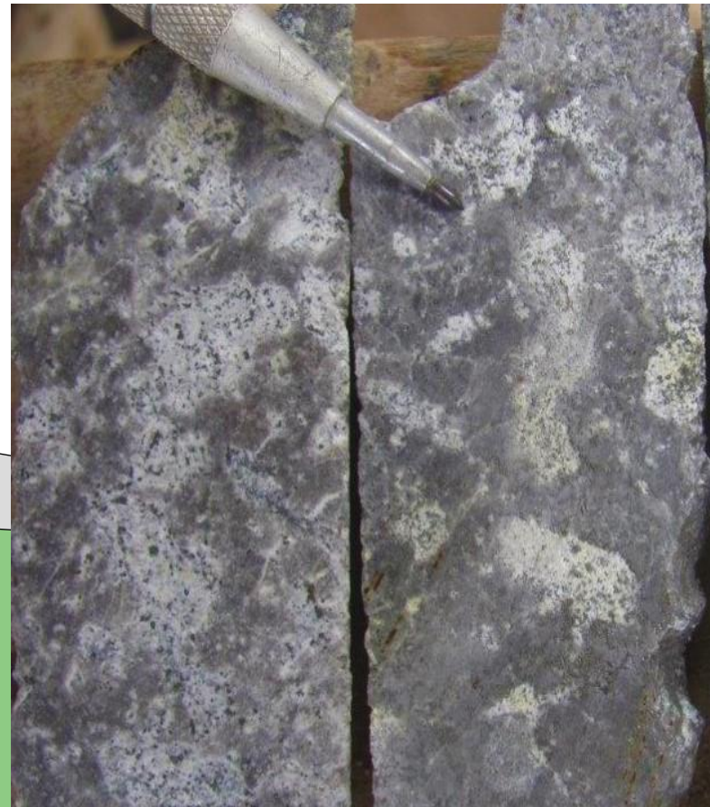
VHD048 at -900m RL, Patchy Texture in Polymictic Breccia (Quartz-diaspore-pyrophyllite-alunite alteration)
