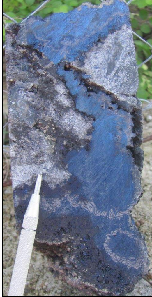
VHD 072 359m: Covellite-pyrite-nukundamite; 29% Cu, 0.07 g/t Au / 1m
