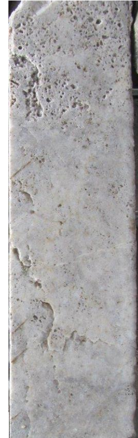
VHD041 at 492m Silicified vuggy residual quartz
