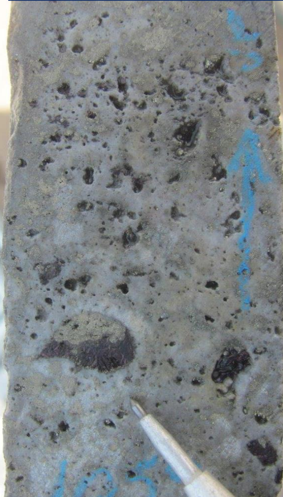
VHD 045 1059m: Covellite-pyrite in VRQ 1.7 % Cu, 0.64g/t Au
