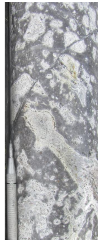
VHD078 at 585m Qu-K- alunite alteration: patchy textures in polymictic breccia
