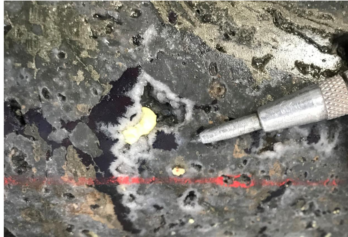
VHD089 378m: Covellite-alunite-native sulphur in vug in vuggy quartz
