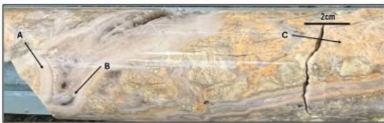
Figure 4: Cockade (A) sulphide banded (B) quartz-adularia (C) veining within the high-grade A-Vein interval reporting 2.8m @ 15.15g/t Au from 59.2m in 25FCDD010.
