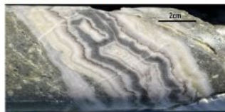
Figure 6: Colloform (A) – crustiform (B) quartz-adularia vein with black silica banding in interval from A Vein
