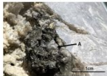
Figure 4: Marcasite vugs (~1% of veined interval, A, D) and marcasite bands (<1% of vein fill, B) can be observed amongst the colloform banded quartz (C) from the A Vein in 25FCDD001.
